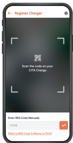
e. Scan the QR code/enter the Charger Serial Number that is pasted on the left side of the charger
